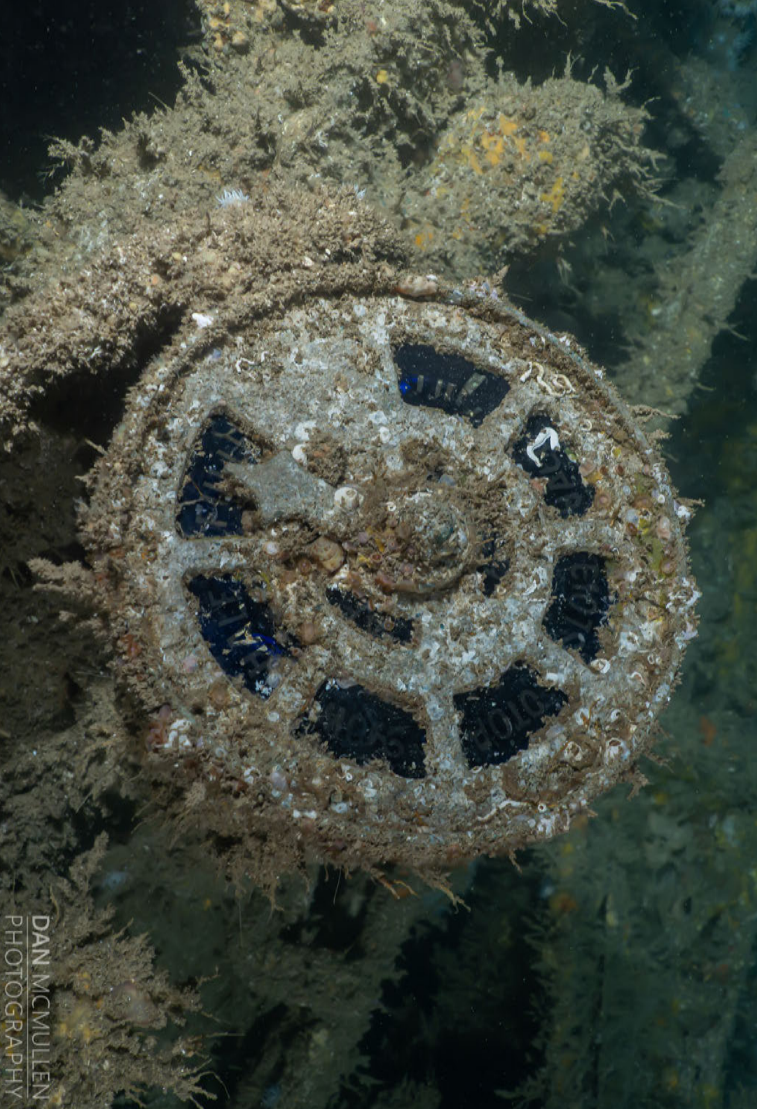
Figure 19: Stern engine revolution telegraph with 7 windows: "Full", "Half", "Slow", "Stop", "Slow", "Half", and "Full". Photo credit: Dan McMullen.
