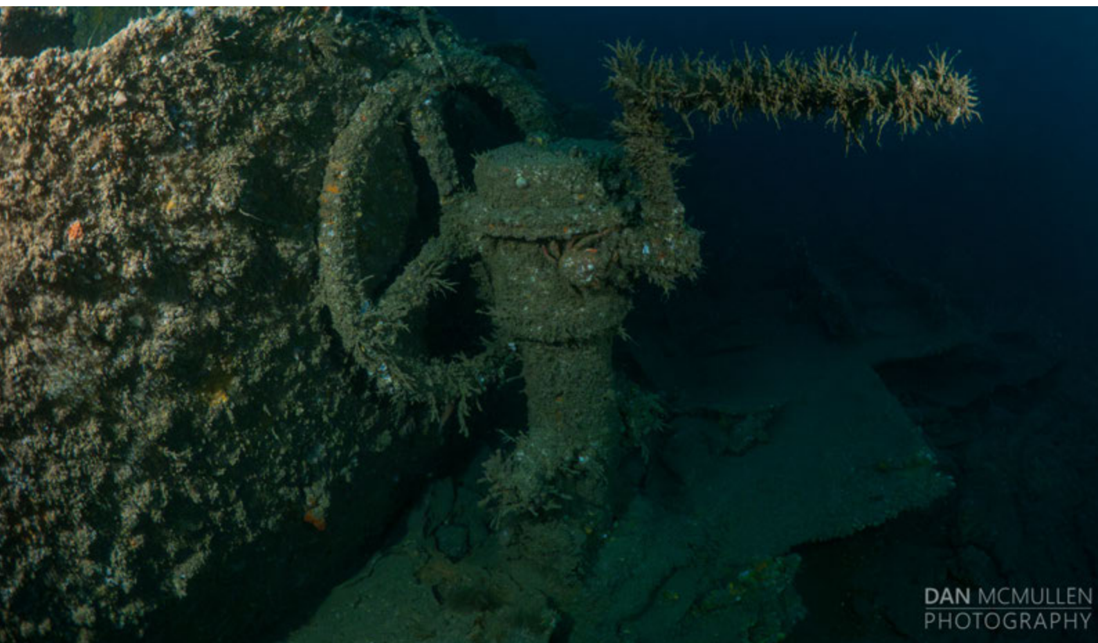
Figure 35: The 1 st "Normand" boiler on the bow section of Tiger with the distinctive three-drum design consisting of a steam drum above two water drums in a triangular layout, with water tubes filling in the two sides of the triangle. Photo credit: Dan McMullen. Figure 36: 5-inch pump around compartments 49 to 50 on the bow section. Photo credit: Dan McMullen.
