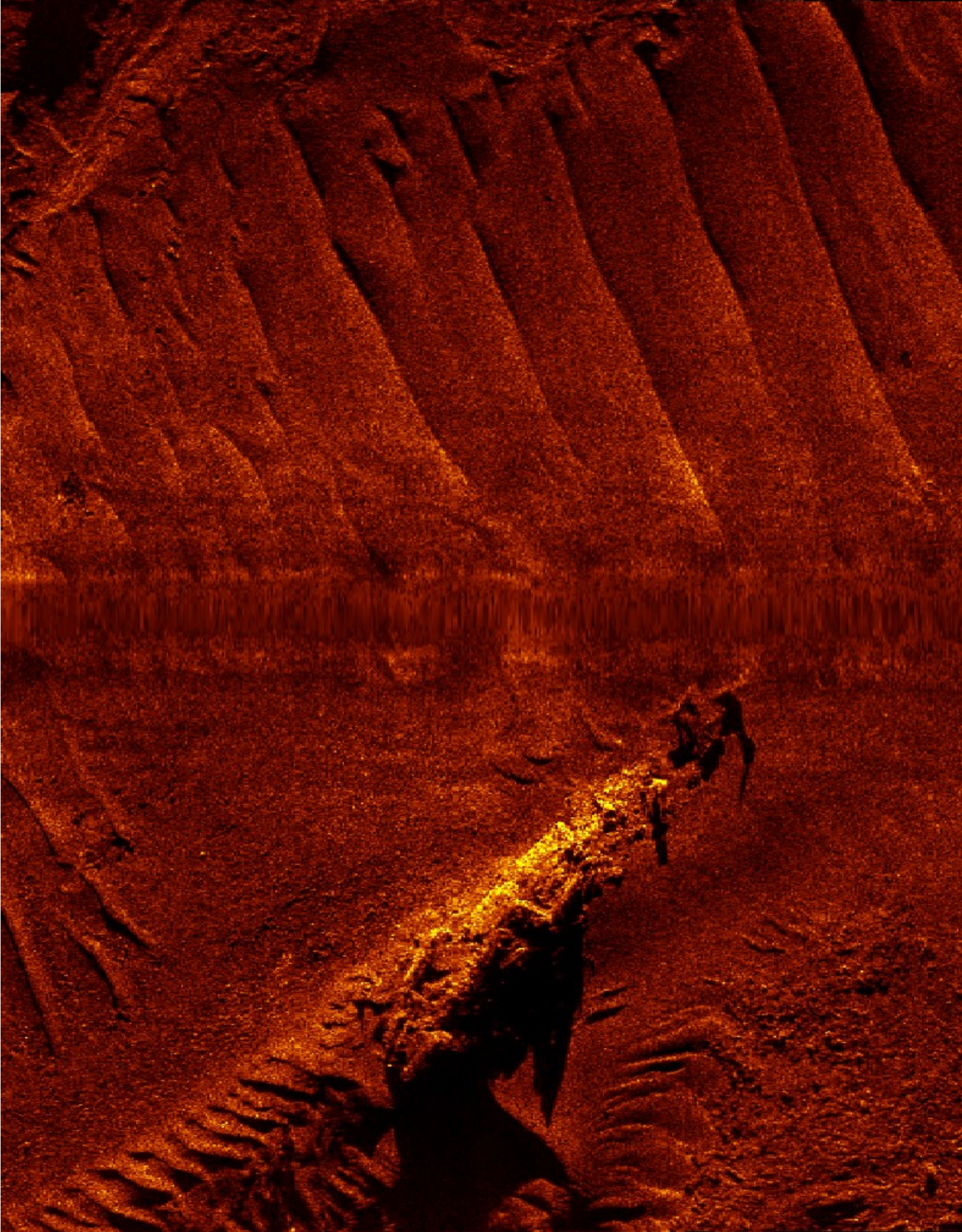
Figure 12 above: Stern section on 780kHz at 37.5m range scanned on 24 July 2026. The horizontal tiller above the well-preserved rudder assembly (top right) casts a long thin shadow on the port side of the wreck. Photo credit: Leo Fielding.
