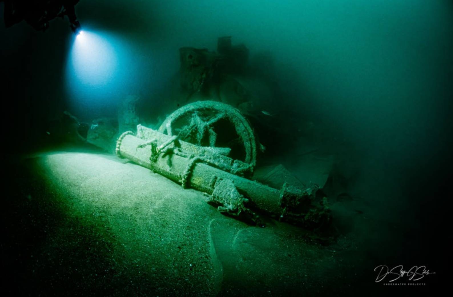
Figure 30 (above): The midships torpedo tube was photographed just in front of the break around compartment number 69. The torpedo tube and slew ring were both fully intact. Photo credit: Dr Steffen G Scholz.
