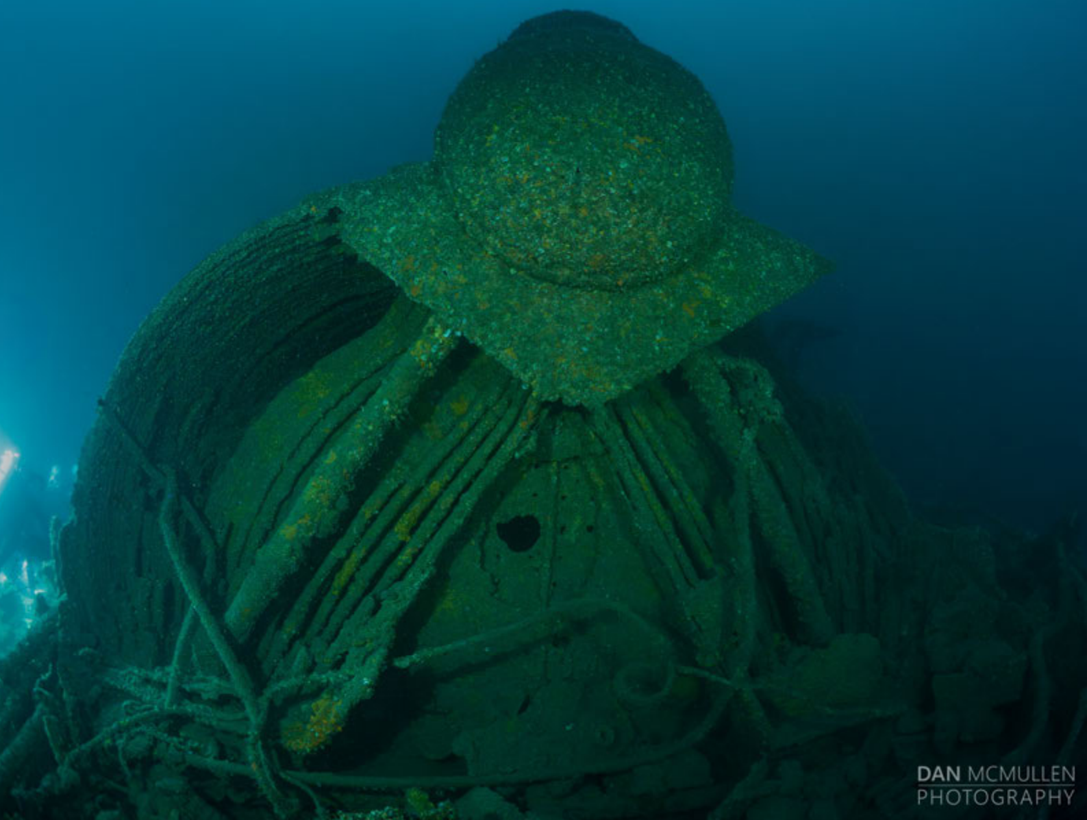
Figure 35: The 1 st "Normand" boiler on the bow section of Tiger with the distinctive three-drum design consisting of a steam drum above two water drums in a triangular layout, with water tubes filling in the two sides of the triangle. Photo credit: Dan McMullen. Figure 36: 5-inch pump around compartments 49 to 50 on the bow section. Photo credit: Dan McMullen.
